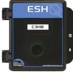
The ESH-A Remote Sensor offers flexible location monitoring of combustible or PID TVOC gases in non-hazardous, non-explosion rated, commercial and light industrial applications. It communicates with a controller or transmitter using current loop into a 100 ohm load or a voltage signal of 0.40 to 2 volts. It can be located at a maximum distance of 200 meters from the controller or transmitter.
