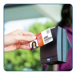
iCLASS SE readers include Open Supervised Device Protocol (OSDP), a new Security Industry Association (SIA) standard that together with Secure Channel Protocol (SCP) provides secure communications and central management.
