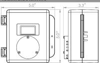
Note: Drawings above are shown with an optional splash guard. Without splash guard, thickness of unit is 71 mm (2.8").
