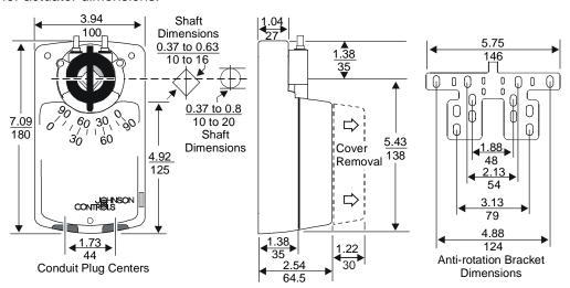
Figure 2: Actuator and Anti-rotation Bracket Dimensions, in. (mm)
