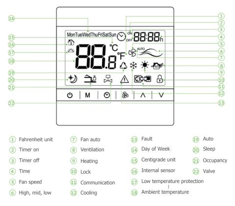
The M button on the front panel for the 2-pipe solution selects the thermostat mode: heating, cooling and ventilation only. The 4-pipe models offer the heating and cooling AUTO mode.
