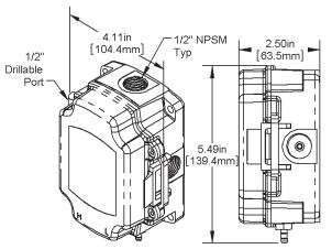
\*BAPI recommends that you do not run wiring for the pressure transmitter in the same conduit as line voltage wiring or with wiring used to supply highly inductive loads such as motors, generators and coils.
