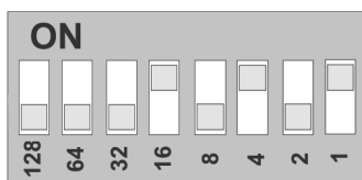
Figure 9: Device address DIP switch block set to address 21
