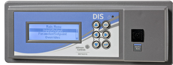
Figure 1: Local Controller Display
