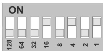
Figure 10: Device address DIP switch block set to Address 21
