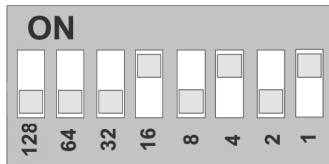
Figure 8: Device address DIP switch block set to address 21
