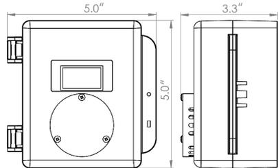
Note: Drawings above are shown with an optional splash guard. Without splash guard, thickness of unit is 71 mm (2.8").
