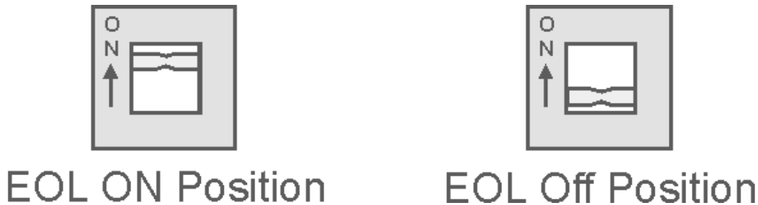
Figure 10: EOL switch positions
