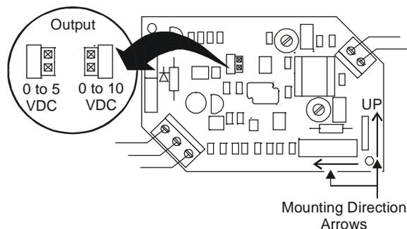
**Figure 1: Mounting Direction Arrows and Output Jumper Location**
